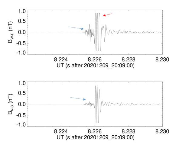
Sferics waveforms belonging to the elves producing stroke occurring on 9/12/2020 at 20:09:08.216501 (43.3942N, 15.4565 S) with a peak current of -639 kA as recorded by two perpendicular magnetic field SGO loops. The blue arrows shows the signatures of the lightning initiation, the red arrow identifies the saturation of the W-E antenna by strong ionospheric sky waves.
