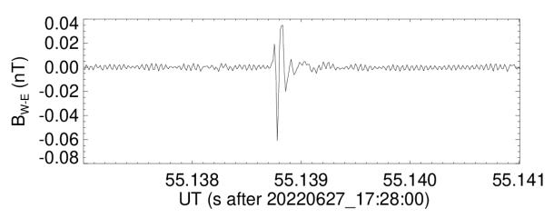
An isolated positive narrow bipolar event as seen by the W-E SGO magnetic loop. According to the ENTLN network this intracloud discharge occurred on 27/06/2022 at 17:28:55.133423 (55.5559N, 11.6501E) with a peak current of 16.27 kA.
